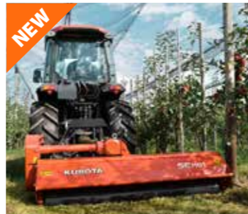
NEW Kubota SE1181 1.8m rear mounted flail mower
