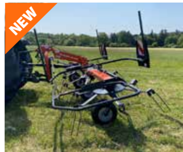
NEW Kubota TE4052 5.2m, 4 rotor tedder, CompactLine model
