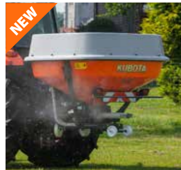
NEW Kubota VS1350H Hydraulic controlled, 1350 litres
