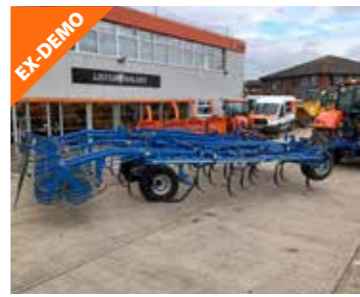
EX-DEMO Köckerling Vario 480 4.8m, 37 tines, hyd. brakes, following harrow
