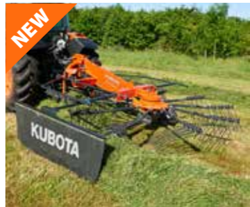
NEW Kubota RA1035 3.5m working width, single rotor rake
