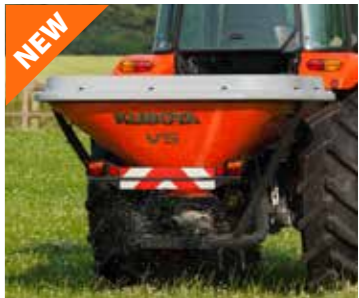
NEW Kubota VS750H Hydraulic controlled, 750 litres
