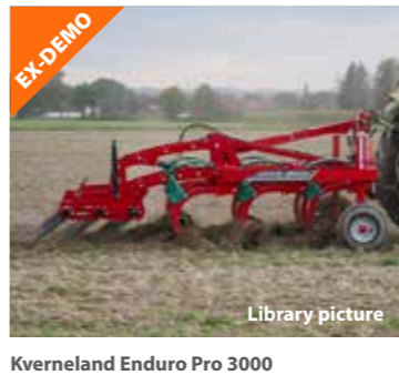
EX-DEMO Kverneland Enduro Pro 3000 3m working width, 3 rows of tines, 10 tines, Triflex 700, available with levelling tines
