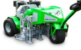
airter® trike 8140 2040 x 1330 x 1400mm (L x W x H) 475kg 8 with working depth from 8 -20cm 8 pointed injection nozzles with 3 air outlets 160cm 1.0km/h 1,200m<sup>2</sup>/h Self-propelled with engine power: 14hp Pneumatic Output 1 x 1,000l/min, 8 - 9 bar Performance: 32 bit
